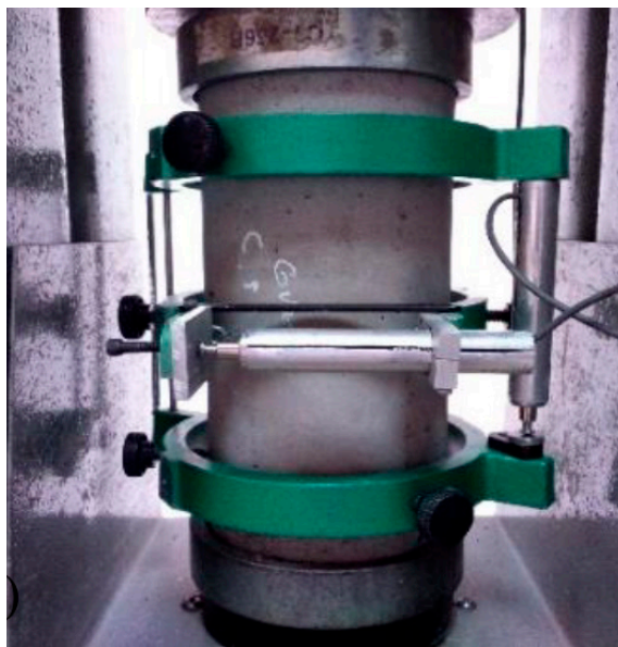
Fig. 1. Test setup: (a) elasticity modulus and Poisson’s ratio, (b) flexural performance of slabs.
